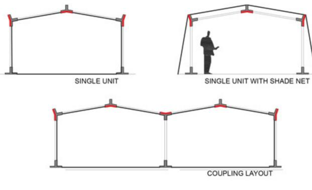
The idea is to create a 5-ways joint in order to have always the same connector, turned depending on the position inside the structure. In fact the hinge has different angles based on its location: when it is used as link between the column and the roof it has a different inclination in front of the connection on the roof top. When positioned in the connection wall-roof, the free way is used as an antenna for the shade net, eliminating the necessity of an extra framework to bear it.
