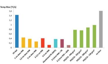
compared with the currently used polyester/cotton tent fabrics. This laminate really outperforms the currently used cladding materials as can be seen in graph 1.
